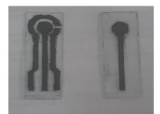
Fig. (6): Different screen-printed electrode based on carrageenan biopolymer
