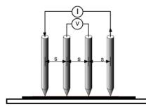
Fig. (3): The 4-point probe with tip
